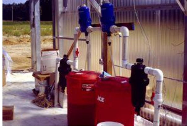
Figure 4. Dual tanks and injectors ensure that chemicals will stay concentrated in the solution.
